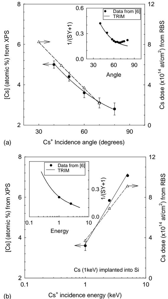
Fig. 1. XPS and RBS defined Cs concentrations as a function of (a)  $\text{Cs}^+$  incident angle at  $1$  keV impact and (b)  $\text{Cs}^+$  impact energy at  $60^\circ$  incidence. In the insets the Cs concentrations derived via the sputter yield relation using both experimentally derived [6] and simulated sputter yields are shown.
