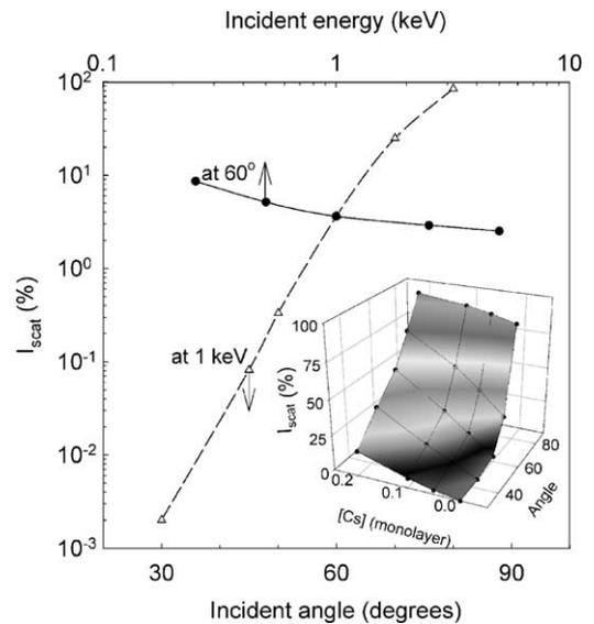
Fig. 3. MARLOWE simulations of the scattering coefficient of  $\text{Cs}^+$  primary ions,  $I_{\text{scatt}}$ , as a function of impact angle (energy fixed at 1 keV) and incident energy (angle fixed at  $60^\circ$ ). In the inset is shown how these vary with increasing Cs coverage.
